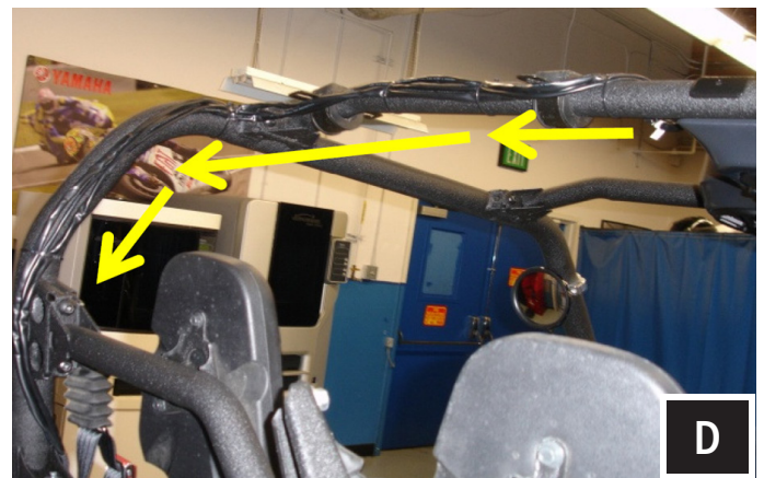
D. After the overhead is installed route the cables down the driver side rear of the vehicle cage, If you choose to run down the front of the cage to avoid removing panels you will not need to use the provided power/ground extension. Using the zip ties provided secure the cables to the cage, be sure to avoid any moving parts and check clearance on the dump bed prior to finalizing any wiring.
