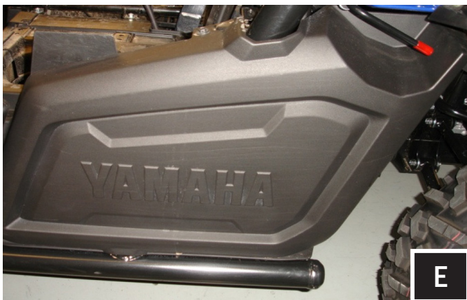
E. Removing the side panel will make running the wiring much easier, there are 3-10mm bolts and 4 plastic fasteners holding this panel.
