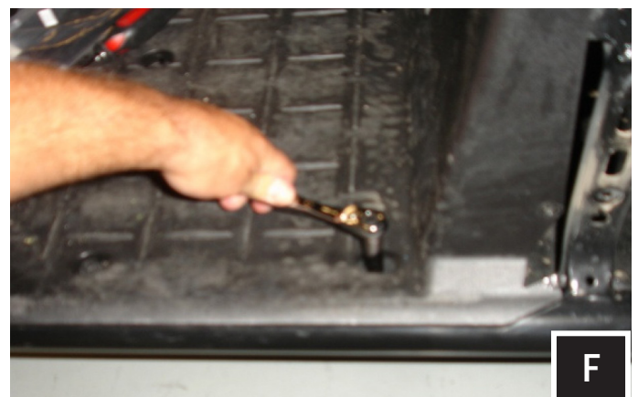
F. After removing the side panel, remove the 2-10mm bolts from the floor
