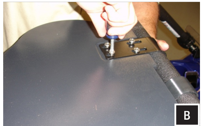
B. Place the stereo in the cage from the interior of the vehicle (speakers toward the front) and loosely install the 4 brackets using the hardware provided, thread locker can be used on the screws for additional security.
